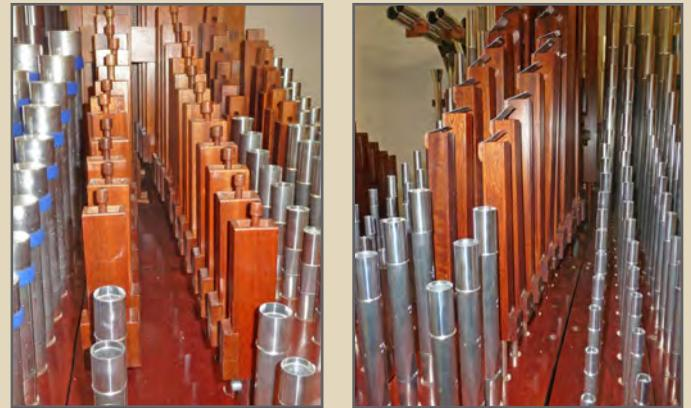
All reed and flue pipes have been manufactured with the finest materials, with alloys ranging from 30% tin for the flutes to 95% tin for the larger 8' and 16' pipes. In-house manufacturing ensures perfect customization to meet tonal and acoustical challenges.
